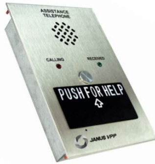
Part #: T1250S Dimensions: 9" H x 6" W x 1.75" D Weight: 3.5 lbs. Material: 13 ga (0.090") brushed stainless steel
